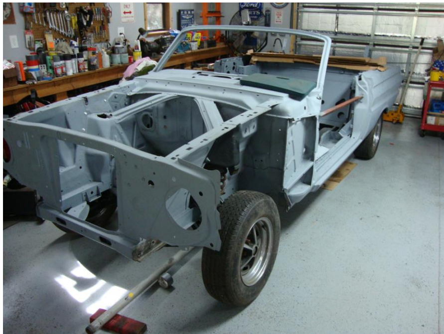
After blasting was completed all surfaces were primed
